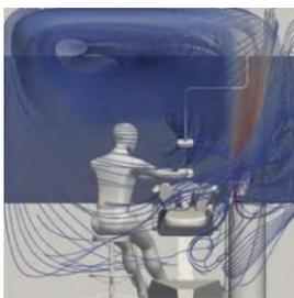
Laminar air flow refers to air flow within the room being both uniform in velocity and direction.
